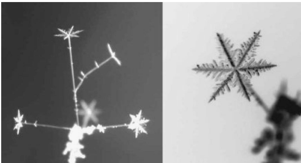
FIG. 3. Group of five ice crystal needles (left), grown along the [0001] axis at -5^\circ\text{C} using an applied potential above threshold. After the needles grew to approximately 1 cm in length, the electric potential was turned off and the crystals were lowered to -15^\circ\text{C} in the diffusion chamber, which is the temperature at which platelike dendrites form. This resulted in the growth of normal single-crystal dendritic stars at the needle ends; one of these is shown as a negative image at right, which has a diameter of 2.4 mm.
